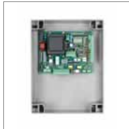
230 Vac control panel with built-in 433.92 Mhz 64-code receiver, integrated display and a number of operating logics. Inputs to connect the encoder (for full features see page 152)
